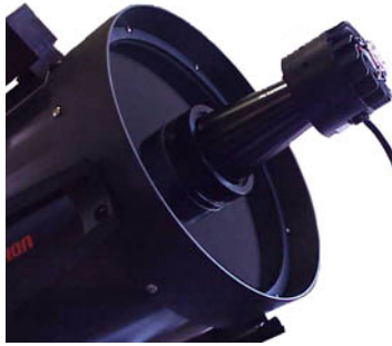
CCD Attached with HyperStar
